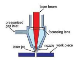
During the laser cutting process, a beam of high-density light energy is focused through a tiny hole of the nozzle. When this **beam** strikes the surface of the work piece, the **material** of the work piece is cut immediately.
