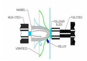
considerable savings in materials and machining when compared to cast or forged parts. Spinning also makes it possible to produce components with thinner wall thicknesses directly, without machining them down to size.
